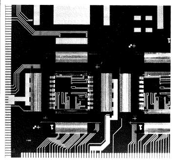
TAB'd Thermal Test Chip in Multichip Module Test Substrate. From IEMT'91. (Photo courtesy Paul Wesling.)
