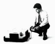
New for 1991 are completely redesigned servo amps, error checking RS-232 communication protocol with selectable 9600/38.4K baud, dual bumper inputs, an enhanced command set, and more.
