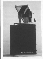
The **ORS-1** is an eyesafe, infrared optical rangefinder specifically designed for mobile robots.
